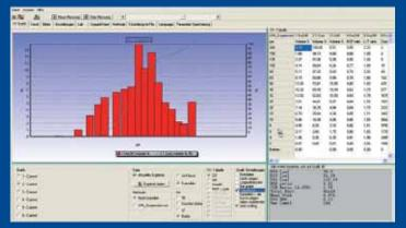
The Microtrac S3500 SI software provides results on particle size by length, width, area, circumference and particle shape. The software also provides for the presentation of data on a wide range of shape properties like aspect ratio, ellipse ratio, compactness, roundness, circularity, concavity and convexity. The data can be exported in either ASCII, Excel or HTML formats. Users can select different report formats.
