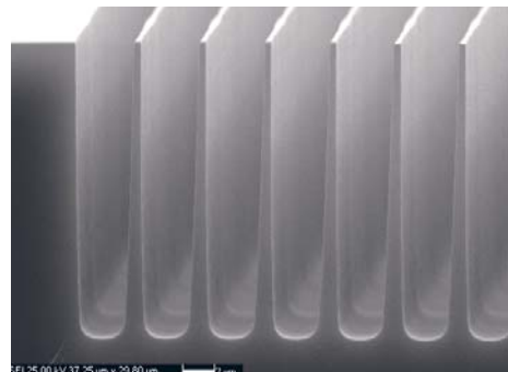
SEM micrograph of high aspect ratio stamp, ratio 34:1
