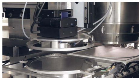
The 6 inch system for Nano Imprint Lithography has been developed for industrial test production, and process optimization purposes.
