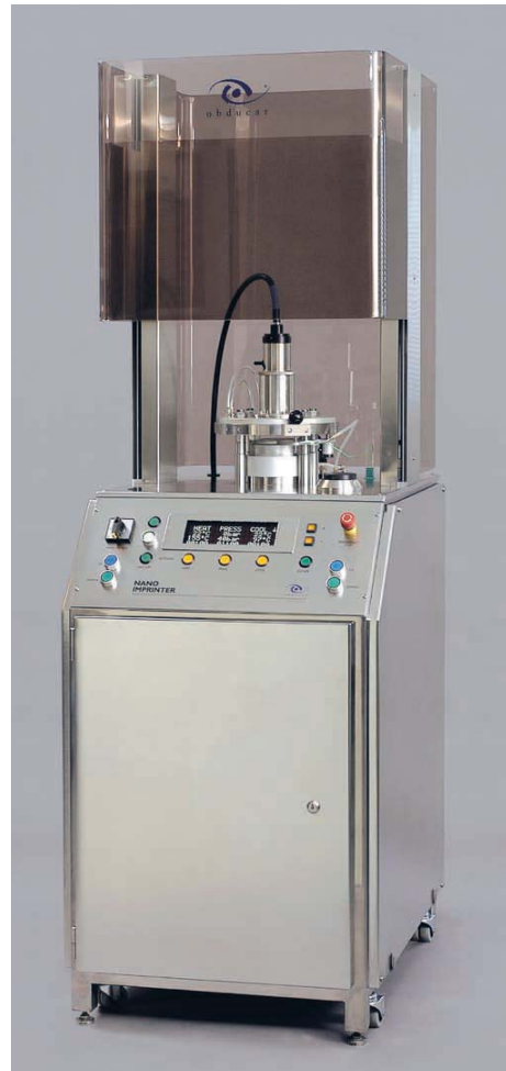
Obducat's 2.5 inch NIL system is developed for R&D purposes.
