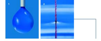
Suspended liquid drop to be evaluated with the Pendant Drop method
