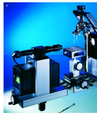
well as in the tilting stages for measuring the contact angle hysteresis. They are connected to the basic unit in seconds and are immediately ready for use. Via a flexible and quick bus system a master controller monitors the communication between the individual system components and of course, the correct timing. The OCA electronics can always be extended by adding new components. At DataPhysics, we take the Plug and Play principle seriously.
