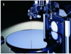
3 SCA 20 and 21 - Contact angle measurement and calculation of the surface free energy of solids 4 Display OCA 10/OCA 20 5 Manual wafer stage WT 200M with multiple dosing unit MD
