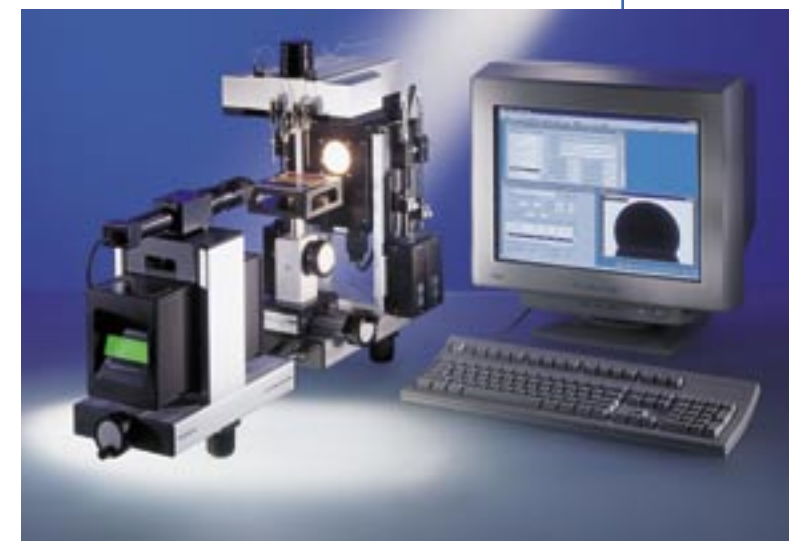
OCA 20 with E-MD/4 electronic dosing system
