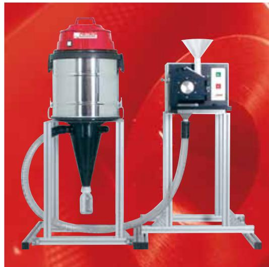
pulverisette 19 with combination-funnel for long- and bulk solids and sample exhauster
