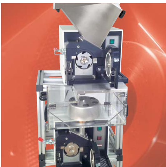
rotor with V-cutting edges and fixed knives
