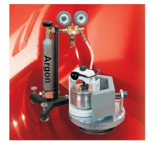
grinding in an inert atmosphere
