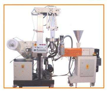
Blown Film Unit 300 with Laboratory Extruder
