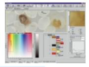
The system is capable of detecting contamination and discoloured powder particles (pink, yellow, brown, black etc.). These irregularities are sorted into different class sizes which are completely user definable. Furthermore, it is possible to define alarm limits. If these are exceeded, a floating contact is activated.
